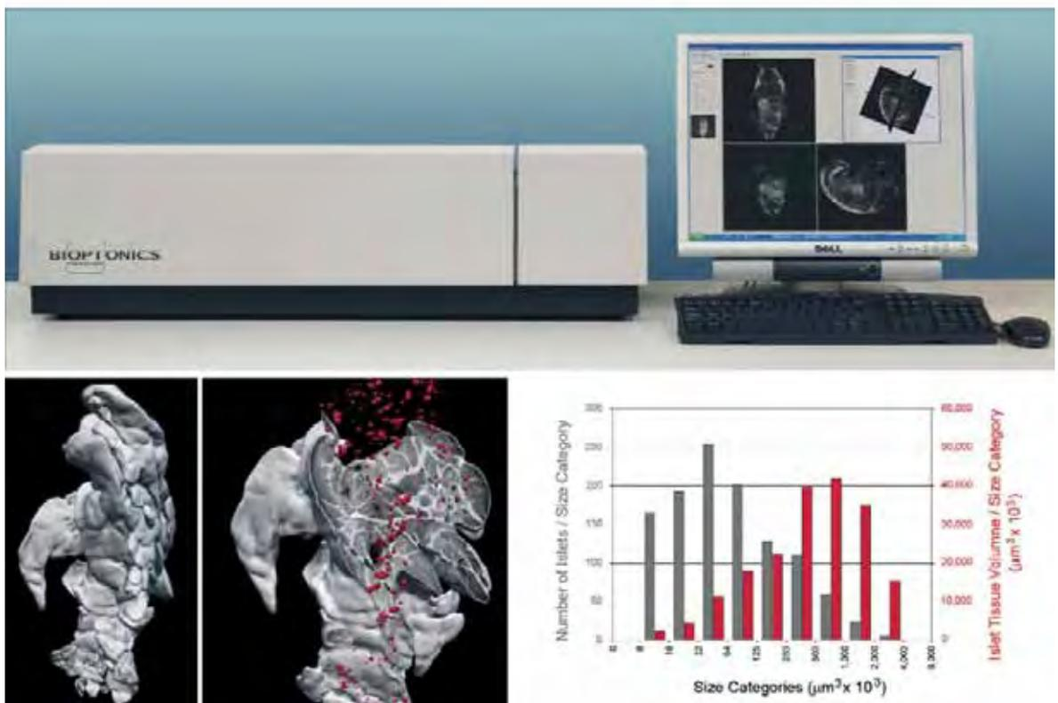
**Figure 1:** Top: We have worked closely with the MRC to design a commercial version of the scanner. Bottom row: OPT scans of a whole adult mouse pancreas (left) which has been fluorescently-labelled with antibodies against insulin to highlight the 3D distribution of Islets of Langerhans (centre). This data can be morphometrically quantified to provide statistics on the volumetric size distribution (right) - *Nature Methods* (2007) 4:31-33.
